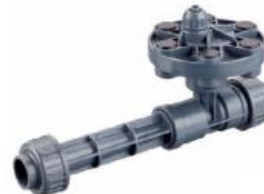
Picture 3: Injector used to create by Venturi effect the vacuum to transport the chlorine gas into the water
